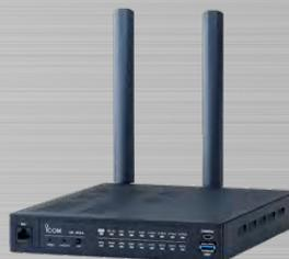
With a VE-PG4 RoIP gateway, the IC-SAT100/M can interconnect with an IP phone, WLAN, LTE, IDAS digital\*2, analog transceivers and other communication systems.
