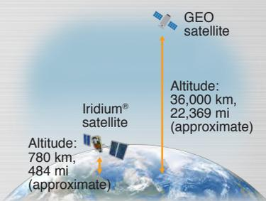
Using 66 Low Earth Orbit (LEO) Iridium® satellites, the IC-SAT100/M provides low-latency communication, and broader, more reliable network coverage, compared to Geosynchronous Equatorial Orbit (GEO) satellites.
