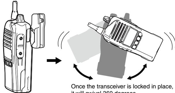
Once the transceiver is locked in place, it will swivel 360 degrees.
