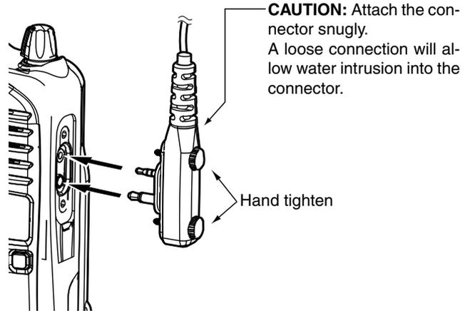
**IMPORTANT:** Keep the [SP MIC] jack cover attached to the transceiver when the speaker-microphone is not in use.
