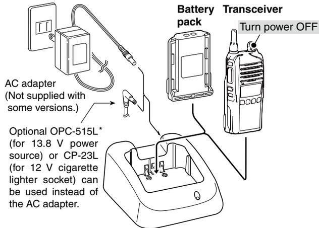
/// **\*CAUTION: NEVER** connect the OPC-515L to a power source using reverse polarity. This will ruin the battery charger.
